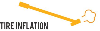
Without a doubt, the single most critical factor for maximizing tire life and minimizing the chance of a catastrophic tire failure is maintaining the proper inflation pressure for a given tire size and load. Once proper tire inflation has been determined, it should be consistently maintained at that level.
